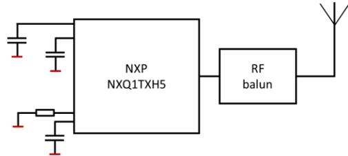
Figure 8: Wireless charging circuit
