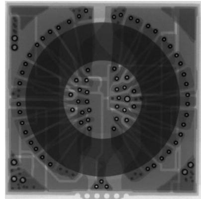
Figure 13: X-Ray of the transformer demonstrator
