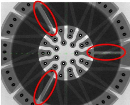
Figure 6: X-Ray of the inductor demonstrator
