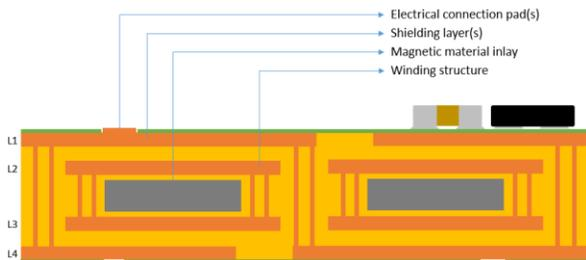
Figure 12: Construction of the transformer demonstrator
