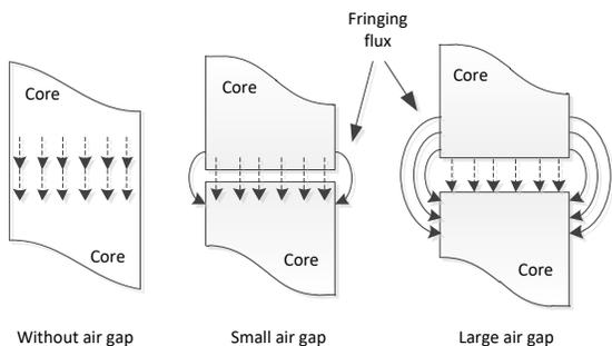
Figure 2: Distribution of magnetic field lines
