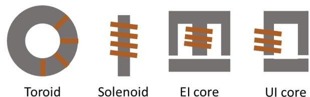
Figure 1: Most common core shapes
