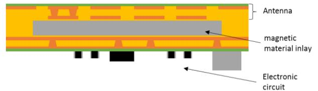
Figure 9: Stack up of PCB
