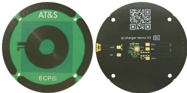
Figure 11: Wireless charging unit with magnetic inlay
