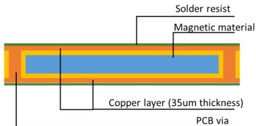
Figure 3: Inductor demonstrator build-up
