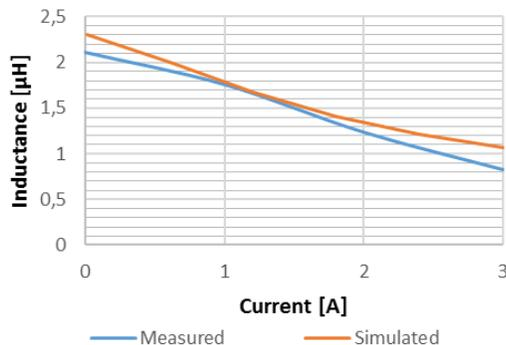
Figure 7: Evaluation results for 3 air gap version
